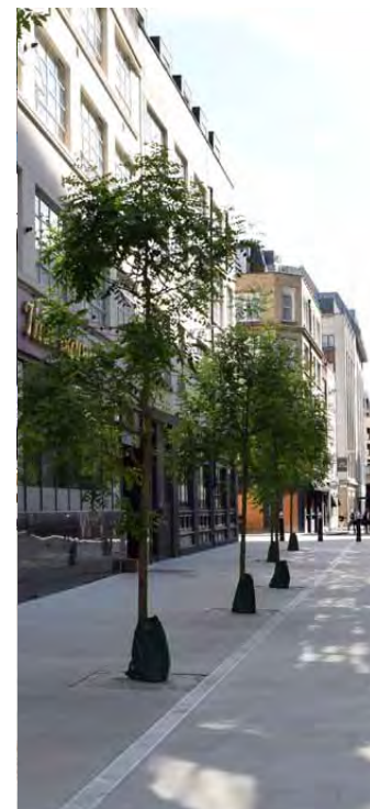
Treegators, as manual tree pit watering provision during establishment
